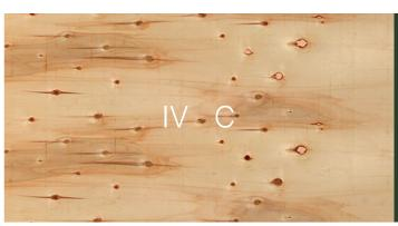
Plywood suitable for packaging or similar uses. All natural wood features (knots, cracks, etc.) are allowed, along with various processing defects, as long as they do not compromise the functionality of the panel (for example: fungus growth and iron/mineral inclusions are not permissible)
