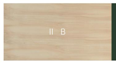
"Natural" face with color variations and sound knots no longer than 10 mm in diameter, suitable for pigmented paints or lacquers. Small knot holes or hairline cracks are allowed, provided they are well-filled patched
