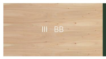
"Closed" face, putty-filled, suitable for uses where face is not visible. Sound, tight knots up to a diameter of 30 mm are allowed; also allowed loose knots, well filled cracks and color variations
