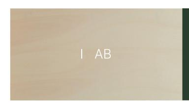
Where face may be visible, ideal for all types of finish (plating, clear varnish, satin finish etc.) Only a few pin knots or sound, tight ones without cracks are allowed. Very small patches, or well-made repairs where color remains consistent with the rest of the surface are also allowed
